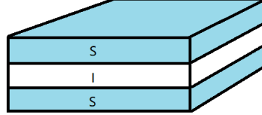
Figure 1: A SIS junction consists of two bulk superconductors separated by a thin insulator layer.
