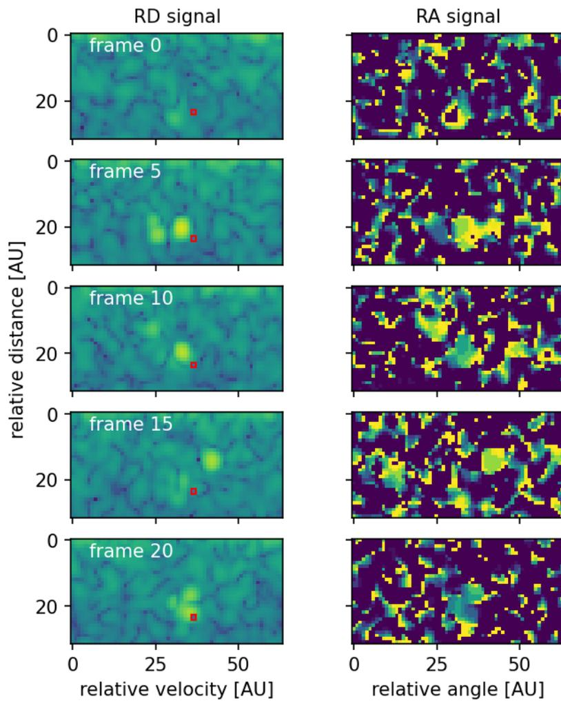
**Figure SUP1:** Range-Doppler and Range-Angle maps for one specific gesture and one-time frame. Apart from noise, one can detect two blobs in the maps, one referring to the person's body gesticulating, and the other to the hand doing the movement. We also marked the voxel with a red box that was used as input for our Skymion Reservoir.
