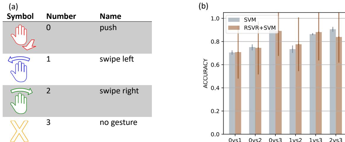
**Figure 3:** a) Table of different hand gestures in data set. b) Comparison detection accuracy between SVM and reservoir plus SVM for different gesture pairs. The error is calculated with the standard deviation of different SVM resulting from the K-Folding.
