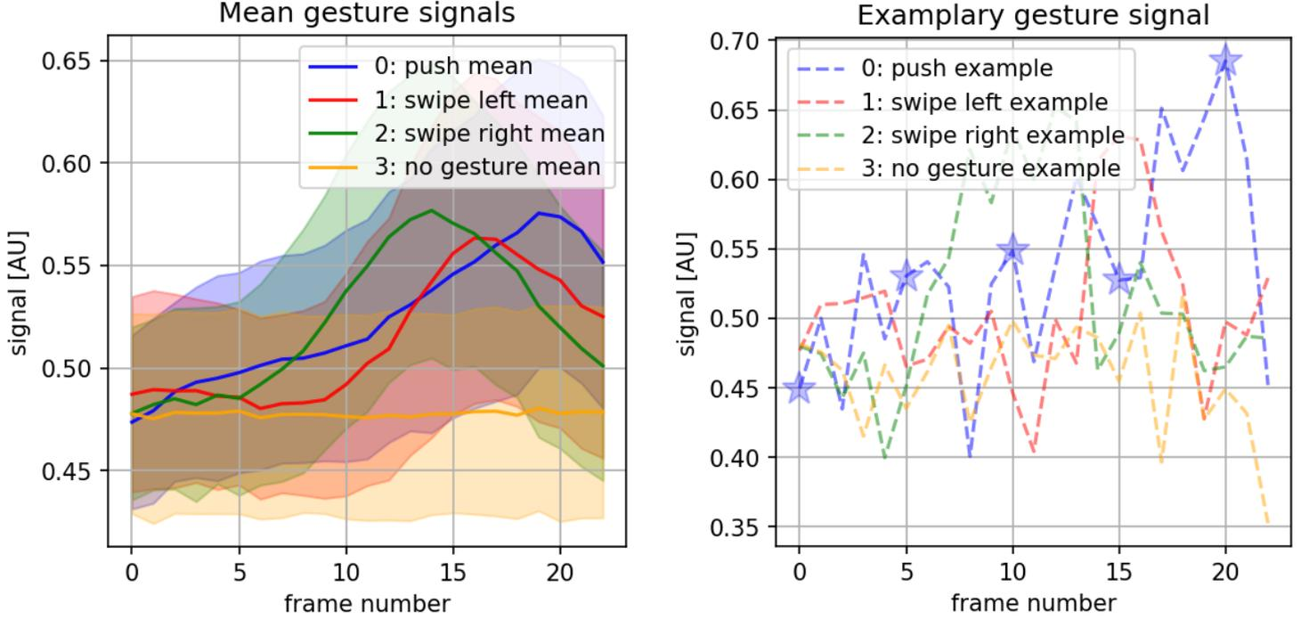
**Figure SUP2** Left: We show the normalized mean signal of every gesture, for the voxel performing best in the Range-Doppler transformed data. Right: Exemplary gestures of every class. The blue star marks the values which are shown in red boxes in Fig. SUP1, which shows the same gesture.
