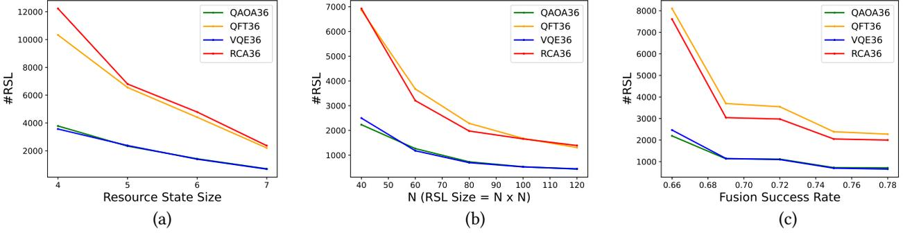
**Figure 10.** Effects of resource state size (a), hardware size (b) and fusion success probability (c), with the resource states being 7-qubit ones for (b)(c), hardware size being 84x84 for (a)(c), and the fusion success probability being 0.75 for (a)(b).
