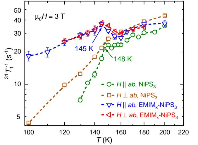
FIG. 10. **Spin-lattice relaxation rates of  $\text{NiPS}_3$  and  $\text{EMIM}_x\text{-NiPS}_3$ .**  $1/^{31}T_1$  shown as a function of temperature, measured with in- and out-of-plane fields of 3 T.
