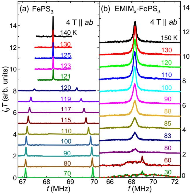
FIG. 4.  $^{31}\text{P}$  NMR spectra of  $\text{FePS}_3$  and  $\text{EMIM}_x\text{-FePS}_3$ . (a) Spectra of  $\text{FePS}_3$  over a range of temperatures above and below  $T_N$ , taken at a fixed in-plane field of 4 T. Successive datasets are offset vertically for clarity. (b) Spectra of  $\text{EMIM}_x\text{-FePS}_3$  taken under the same conditions. The spectral intensities at 30 and 60 K are multiplied by a factor of two; dashed lines represent Gaussian fits to the data.
