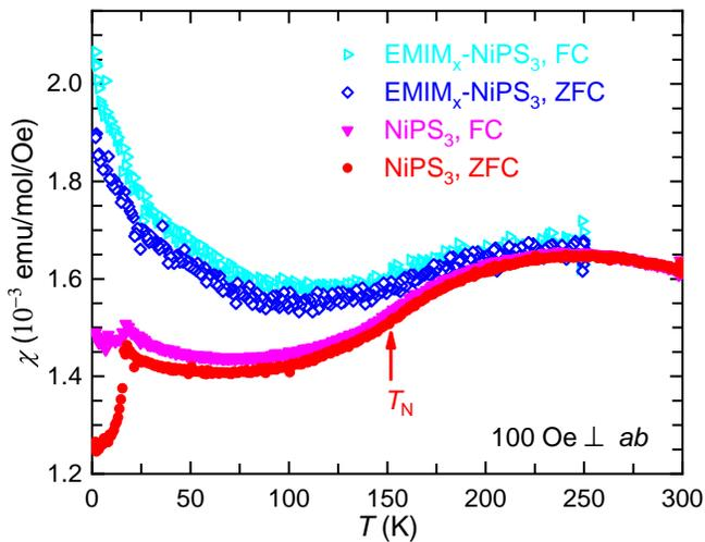
FIG. 7. **Magnetic susceptibility of NiPS<sub>3</sub> and EMIM<sub>x</sub>-NiPS<sub>3</sub>.**  $\chi(T)$  measured in an out-of-plane field of 100 Oe under FC and ZFC conditions.
