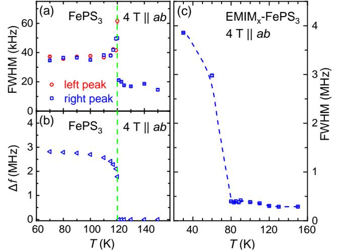
FIG. 5. NMR line widths and splittings in  $\text{FePS}_3$  and  $\text{EMIM}_x\text{-FePS}_3$ . (a) FWHM of the primary spectral peak, or peaks, in  $\text{FePS}_3$  [Fig. 4(a)] shown as a function of temperature. (b) Splitting,  $\Delta f$ , of NMR peaks in  $\text{FePS}_3$  as a function of temperature. (c) FWHM of the broad NMR spectrum of  $\text{EMIM}_x\text{-FePS}_3$  [Fig. 4(b)] shown as a function of temperature.
