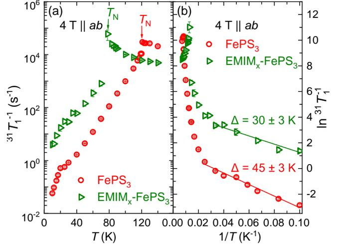
FIG. 6. Spin-lattice relaxation rates of  $\text{FePS}_3$  and  $\text{EMIM}_x\text{-FePS}_3$ . (a)  $1/^{31}T_1$  shown as a function of temperature, measured with an in-plane field of 4 T. (b)  $1/^{31}T_1$  shown in semilog form as a function of  $1/T$ . The straight solid lines represent linear fits to the data in the low-temperature regime.  $\Delta$  is a gap value extracted from the gradient of each line.
