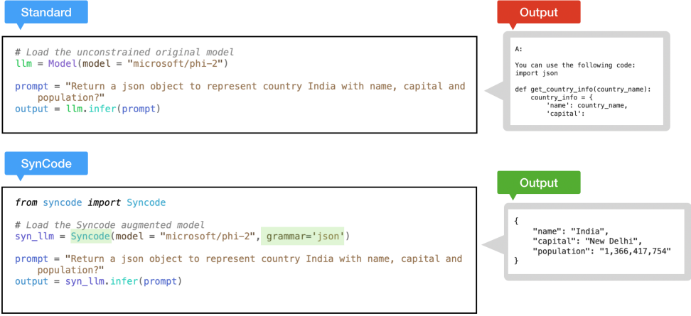
Fig. 9. The upper section displays erroneous output from a standard LLM generation, failing to produce the intended JSON format. The lower segment showcases the fix achieved through the use of the SYNCODE library.
