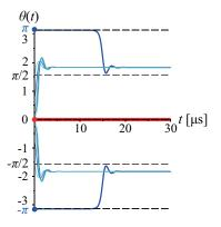
FIG. 6. Plots of the relative phase  $\theta(t)$  as a function of time obtained by numerically solving Eqs. (A7a)-(A7c) for the same parameter values as in Fig. 5 except for  $C_1 = 0$  and  $C_2 = 1$  MHz. The magnitude of  $\varphi$  is bounded as Eq. (D2), and the synchronized precession of the left and the right magnetization,  $\dot{\theta}(t) = 0$ , remains valid. Under the initial condition  $\theta(0) = 0$ , we get  $\varphi = 0$  for  $C_1 = 0$ .
