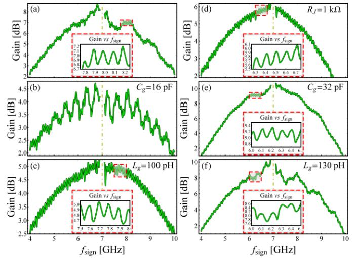
**Fig. 4.** Frequency response of the JTWPA and effect of change of parameters. The signal power is fixed to -100 dBm, the pump frequency to 7 GHz, and power to -55 dBm. The insets detail the gain ripples. The parameters in (a) are as in Table I, while in other panels only one parameter value changes from this table, i.e., (b)  $C_g = 16$  pF, (c)  $C_g = 32$  pF, (d)  $R_J = 1$  k $\Omega$ , (e)  $L_g = 100$  pH, and (f)  $L_g = 130$  pH.
