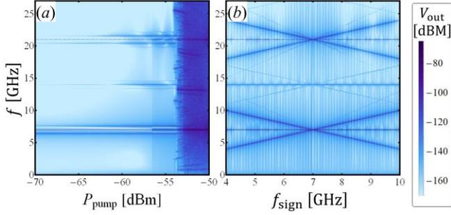
**Fig. 3.** Fourier spectra of the output voltage versus the pump power level for  $f_{sign} = 6.42$  GHz (a) and versus the signal frequency for  $P_{pump} = -55$  dBm (b). The color intensity scale represents the amplitude of the spectral components whose frequency can be read on the left vertical axis. The pump frequency is 7 GHz and the input signal power is -100 dBm.
