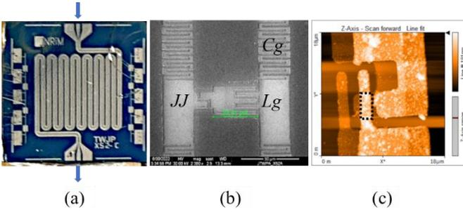
**Fig. 1.** The realized JTWPA: (a) the whole chip; (b) a SEM photograph of a single cell; (c) an AFM picture of one of the 990 JJs forming the JTWPA
