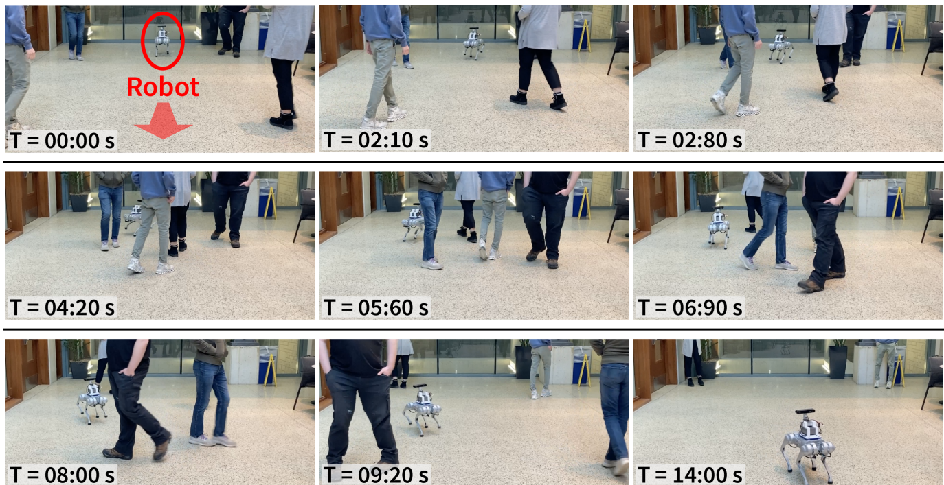
Fig. 12: Snapshots from the real-world demonstration with 4 pedestrians. The specification of this demonstration mimics the simulation tests shown in Figure 9. Videos of the demonstrations are included in the project website: https://sites.google.com/view/brne-crowdnav .
