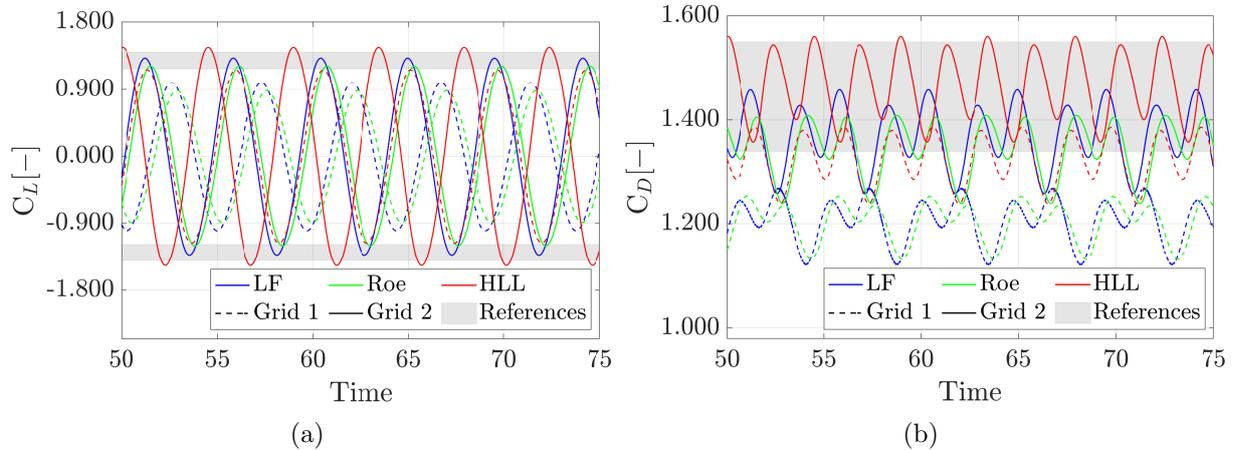
Figure 23: Unsteady turbulent flow past a circular cylinder: (a) Lift and (b) drag coefficients as a function of time for the two meshes and the three convective stabilisations.
