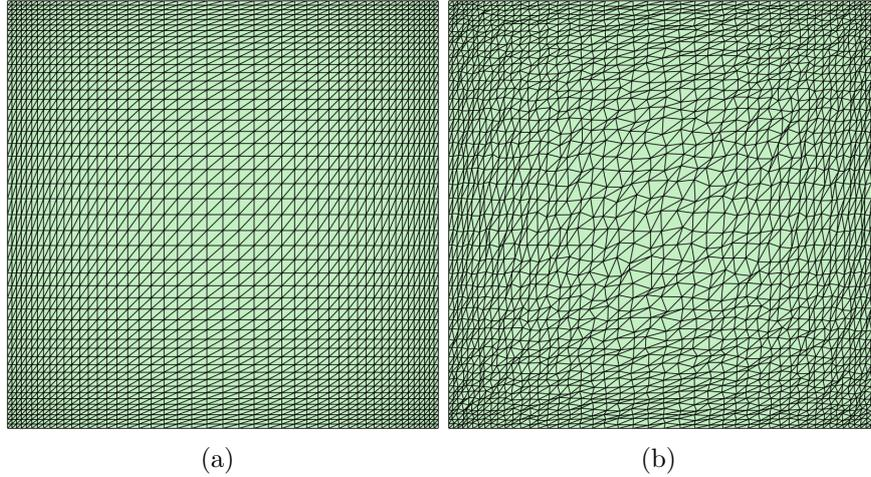
Figure 4: Lid-driven cavity flow: (a) Regular and (b) distorted triangular meshes used for the convergence study.
