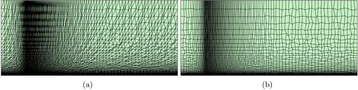
Figure 17: Turbulent flow over a flat plate: Distorted (a) triangular and (b) quadrilateral coarse meshes.
