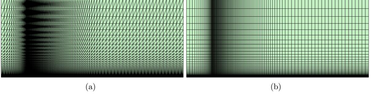
Figure 12: Turbulent flow over a flat plate: (a) Triangular and (b) quadrilateral coarse meshes.
