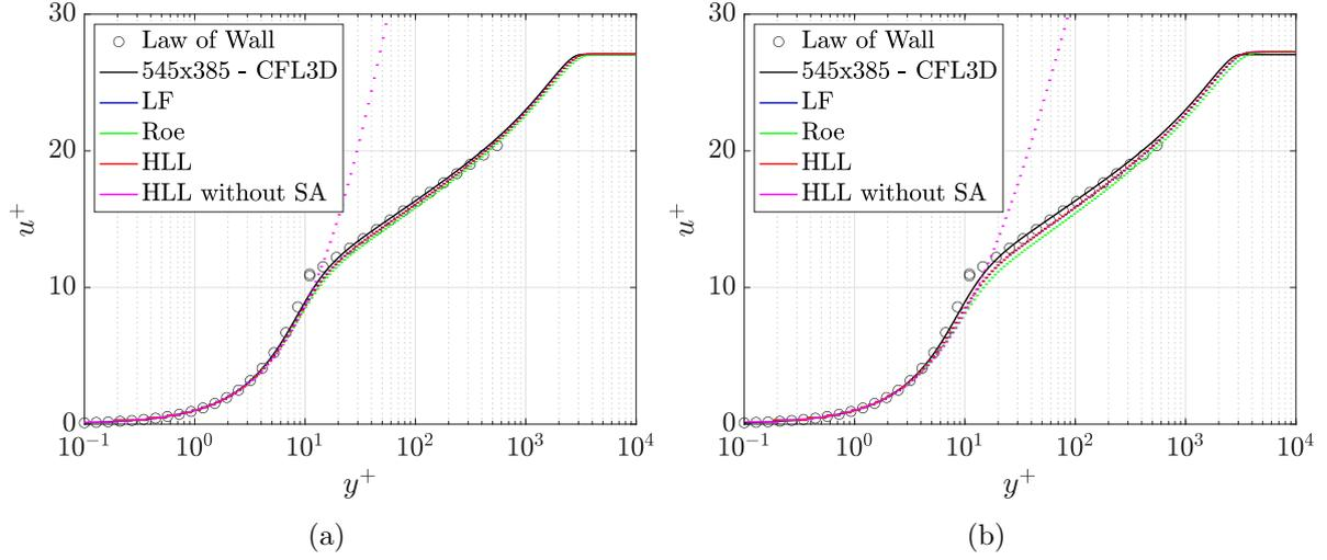
Figure 15: Turbulent flow over a flat plate: Dimensionless value of  $u^+$  as a function of  $y^+$  at  $x_1 = 0.97008$  for (a) the second triangular mesh and (b) the second quadrilateral mesh, compared to the law of wall and a reference numerical solution. The solution for the HLL convective stabilisation without the SA model is also shown.
