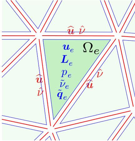
Figure 1: Detail of a triangular mesh highlighting a cell  $\Omega_e$  where the velocity  $\mathbf{u}_e$ , velocity gradient  $\mathbf{L}_e$ , mean pressure  $p_e$ , turbulent variable  $\tilde{v}_e$  and gradient of the turbulent variable  $\tilde{\mathbf{q}}_e$  are defined and internal edges where the hybrid velocity  $\hat{\mathbf{u}}$  and hybrid turbulent variable  $\hat{v}$  are defined.
