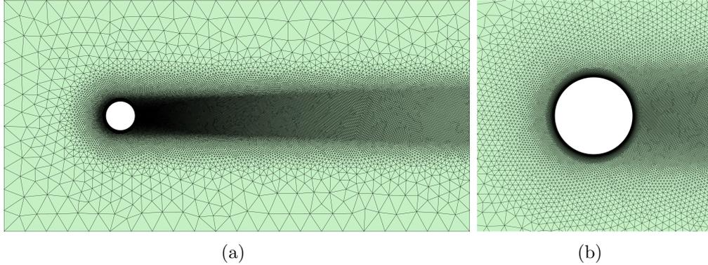
Figure 21: Unsteady turbulent flow past a circular cylinder: (a) Second mesh with 98,193 cells and (b) detail of the inflation layer.
