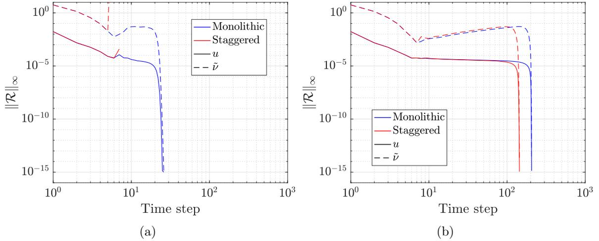
Figure 25: Turbulent flow over a flat plate: Evolution of the residuals with (a)  $\gamma_{\max} = 2$  and (b)  $\gamma_{\max} = 1.2$ .
