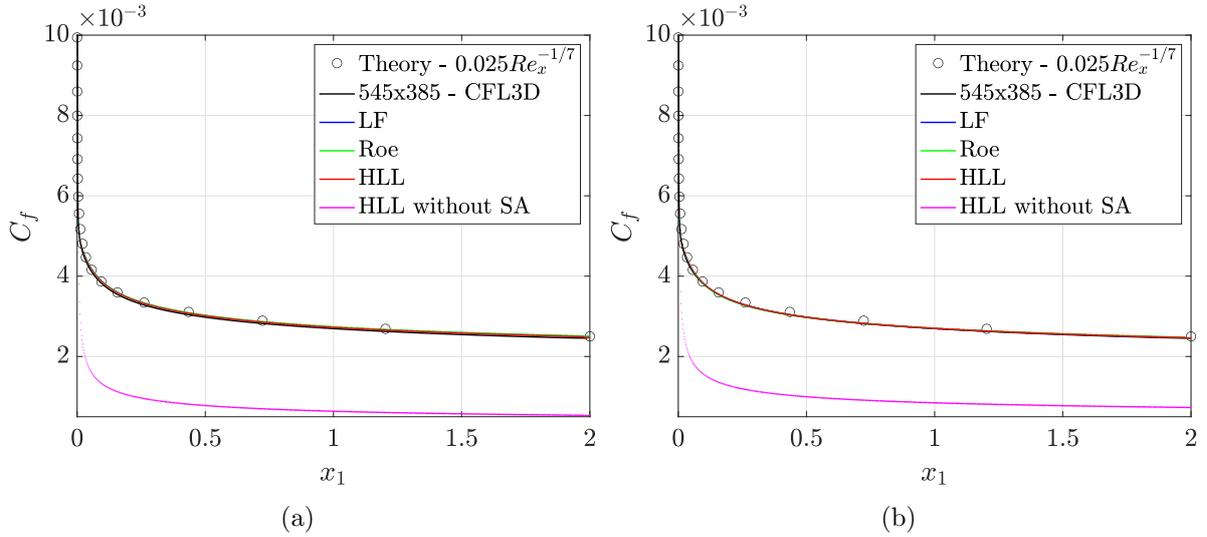
Figure 14: Turbulent flow over a flat plate: Skin friction along the plate for (a) the second triangular mesh and (b) the second quadrilateral mesh, compared to the Blasius solution and a reference numerical solution. The solution for the HLL convective stabilisation without the SA model is also shown.
