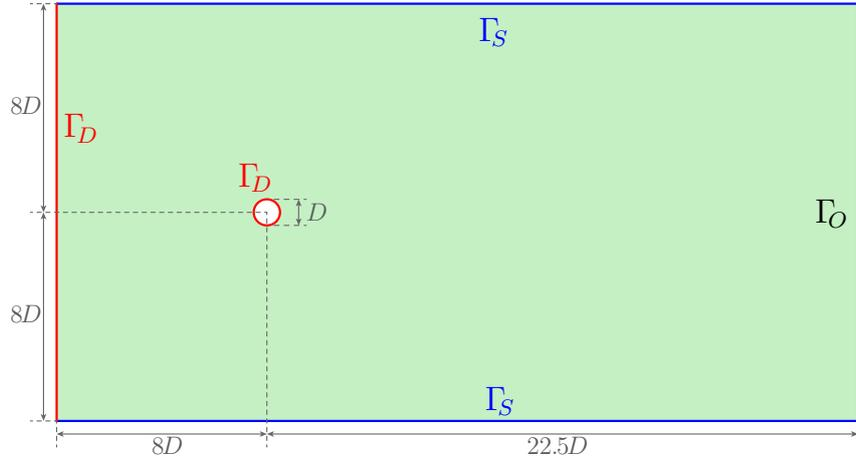
Figure 7: Unsteady laminar flow past a circular cylinder: Problem setup.
