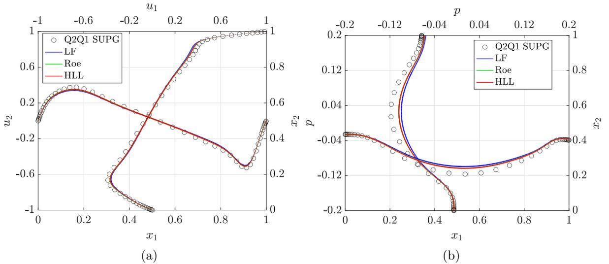
Figure 6: Lid-driven cavity flow: Profiles of (a) velocity and (b) pressure along the centre-lines, using the fourth regular mesh and different convection stabilisations.
