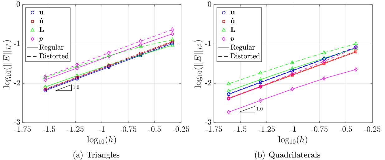
Figure 3: Couette flow: Mesh convergence of the error of the cell velocity, face velocity, gradient of the velocity and pressure for regular and distorted triangular and quadrilateral meshes using the HLL convection stabilisation.
