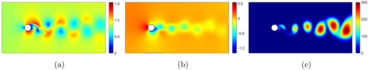
Figure 22: Unsteady turbulent flow past a circular cylinder: Snapshots of the (a) magnitude of the velocity, (b) pressure and (c) turbulent viscosity at  $t = 61$ .
