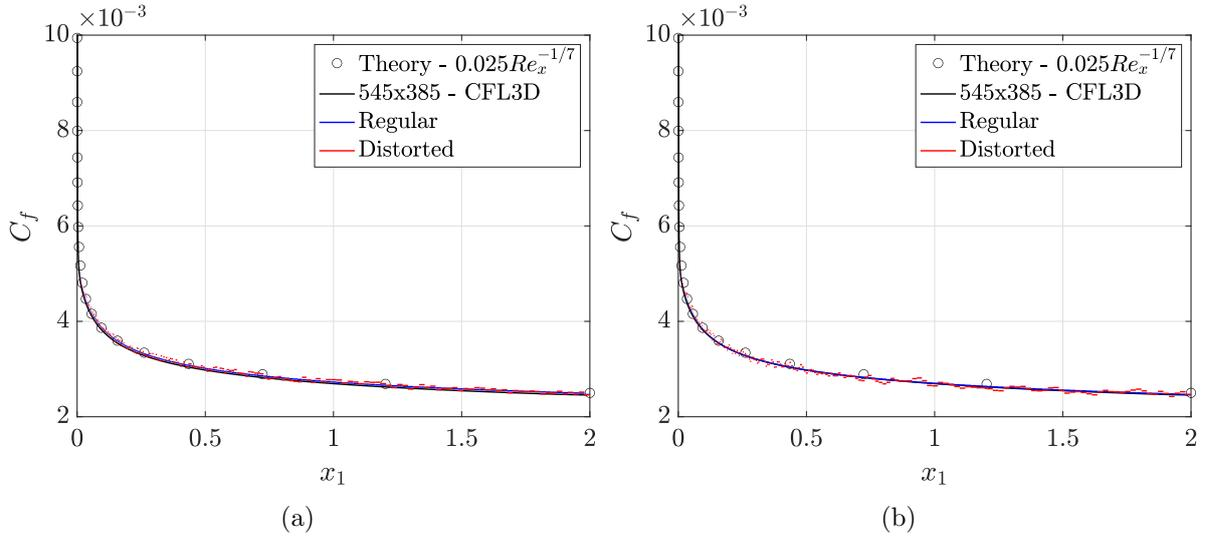
Figure 18: Turbulent flow over a flat plate: Skin friction on the second (a) triangular and (b) quadrilateral distorted meshes compared to the computation with regular meshes, the Blasius solution and a reference numerical solution.
