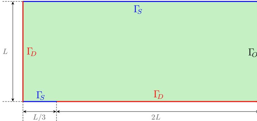
Figure 11: Turbulent flow over a flat plate: Problem setup.
