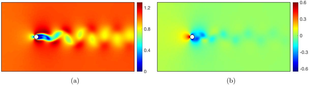
Figure 9: Unsteady laminar flow past a circular cylinder: Snapshots of the (a) magnitude of the velocity and (b) pressure at  $t = 65$ .
