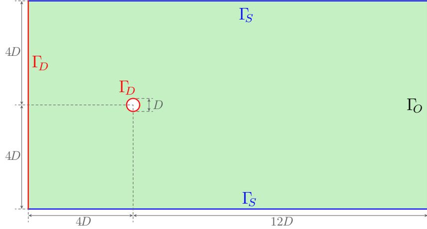
Figure 20: Unsteady turbulent flow past a circular cylinder: Problem setup.
