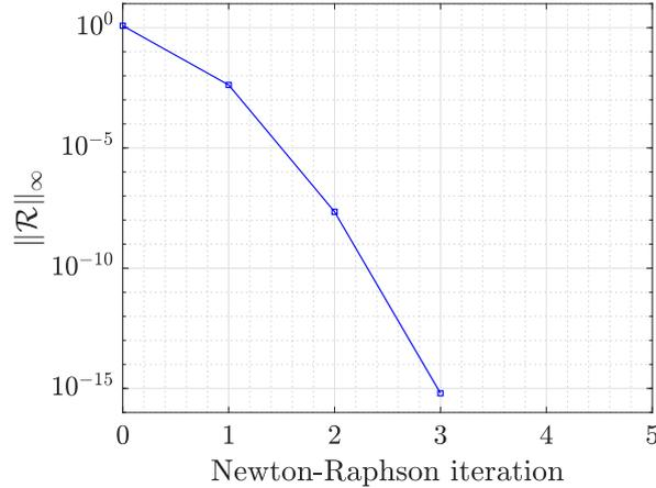
Figure 24: Residual of equation 41 as a function of the number of Newton-Raphson iterations for the Couette example.
