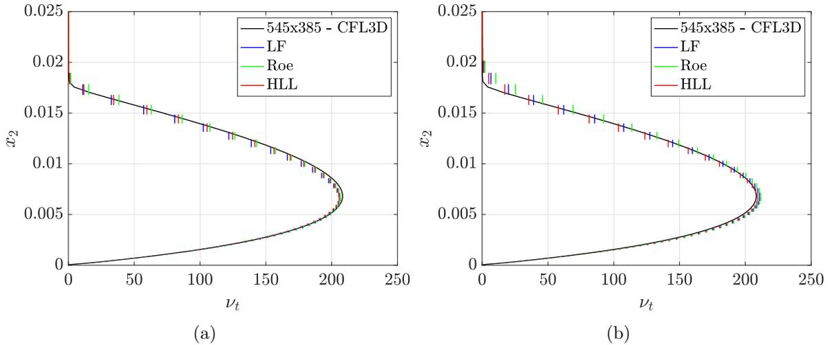
Figure 16: Turbulent flow over a flat plate: Turbulent viscosity at  $x_1 = 0.97008$  for (a) the second triangular mesh and (b) the second quadrilateral mesh, compared to a reference numerical solution.
