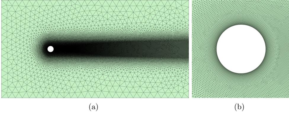
Figure 8: Unsteady laminar flow past a circular cylinder: (a) Second mesh with 135,273 cells and (b) detail of the inflation layer.
