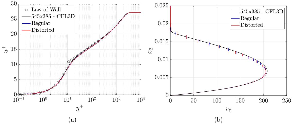
Figure 19: Turbulent flow over a flat plate: (a) Dimensionless value of  $u^+$  as a function of  $y^+$  and (b) turbulent viscosity, at  $x_1 = 0.97008$ , on the second triangular distorted mesh compared to the computation with regular meshes and a reference numerical solution.
