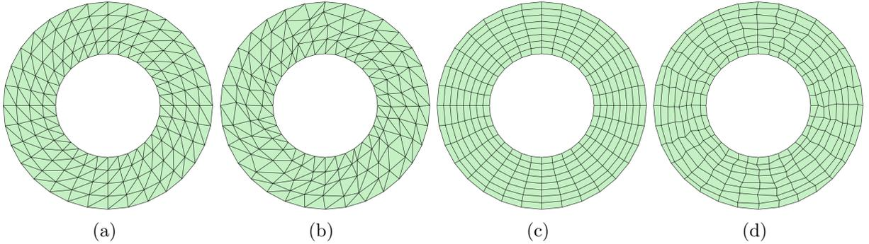
Figure 2: Couette flow: (a,b) Triangular and (c,d) quadrilateral meshes used for the convergence study.
