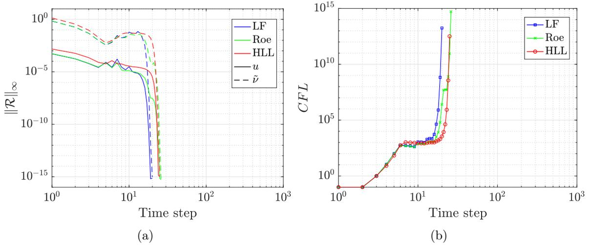
Figure 13: Turbulent flow over a flat plate: Evolution of the (a) residuals and (b) CFL during the pseudo-time marching for the computation using the second quadrilateral mesh.
