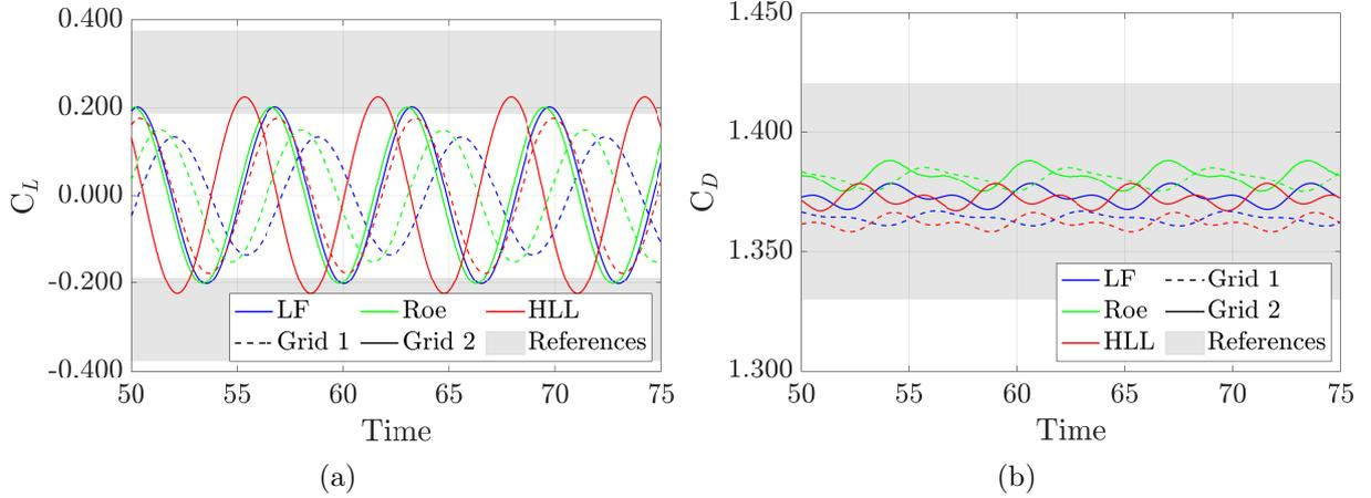
Figure 10: Unsteady laminar flow past a circular cylinder: (a) Lift and (b) drag coefficients as a function of time for the two meshes and the three convective stabilisations.
