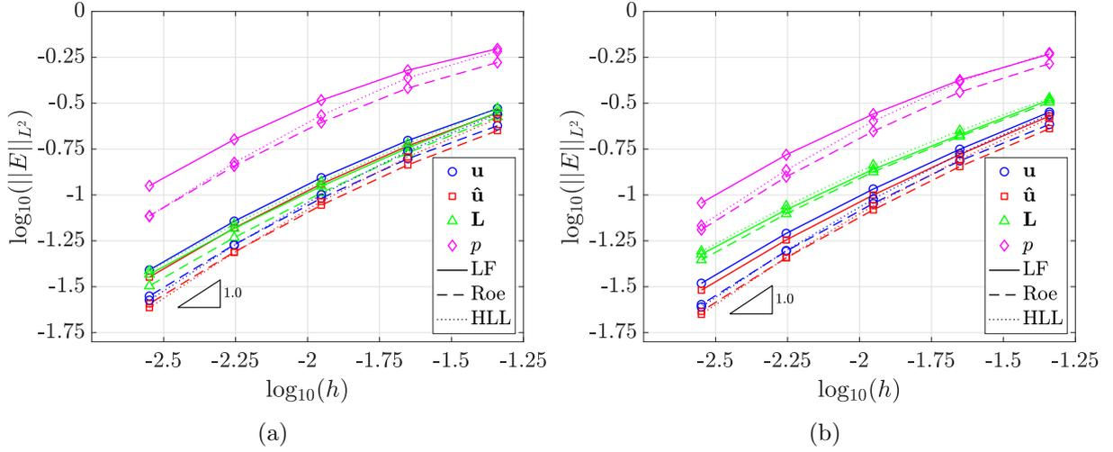
Figure 5: Lid-driven cavity flow: Mesh convergence of the error of the cell velocity, face velocity, gradient of the velocity and pressure for (a) regular and (b) distorted triangular meshes using different convection stabilisations.
