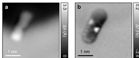
**Figure S9.** (a) In-gap STM image of **1** whose orbital density images are shown in Figure 3 ( $V = 0.2$  V and  $I = 0.5$  pA). (b) Constant-current AFM image acquired simultaneously with (a). The two bright features at the center of **1** in (b) correspond to the strongly-tilted hexagonal rings of the biphenyl moiety.
