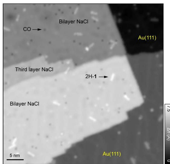
**Figure S1.** Overview STM image of the sample acquired with a gold-terminated tip ( $V = 0.2$  V and  $I = 0.3$  pA). The sample consists of large bilayer NaCl islands on Au(111), a minority of third-layer NaCl islands, carbon monoxide (CO) molecules that appear as circular depressions, and 2H-1 molecules.
