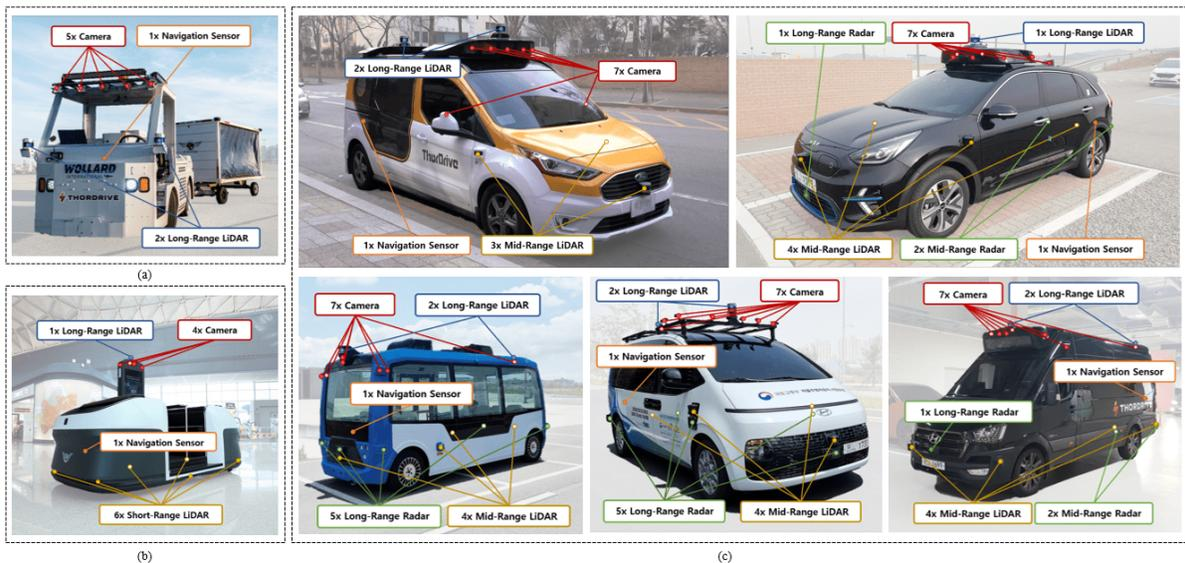
Fig. 2. Developed autonomous driving platforms. (a) Airfields: tow tractor. (b) Crowded indoors: shuttle (AirRide). (c) Urban: top: from the left, last-mile delivery vehicle (Eligo) and on-demand taxi, and bottom: from the left, health care service vehicle, road infra monitoring vehicle, and shuttle.
