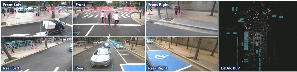
Fig. 5. Object detection results in complex urban environments. The cyan, pink, and purple boxes show a vehicle, a pedestrian, and a cyclist, respectively.
