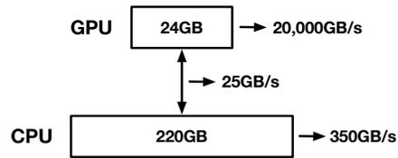
Figure 1. Memory space and processing speed for GPU, CPU, and I/O between CPU and GPU. The speed is tested with OPT-30B MLP Linear on NVIDIA A10 GPU and Intel Xeon @ 2.30GHz CPU, calculated as parameter size divided by processing time.
