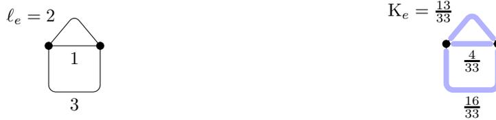
Figure 5: Graph with edge resistances (left) and curvatures (right).
