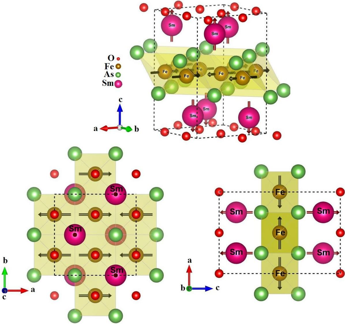
Fig. 1. Crystal and proposed magnetic structure of  $\text{SmFeAsO}$  based on experiment in the temperature range of  $5\text{K} \leq T \leq 110\text{K}$ , shown for a  $\sqrt{2} \times \sqrt{2} \times 1$  supercell.
