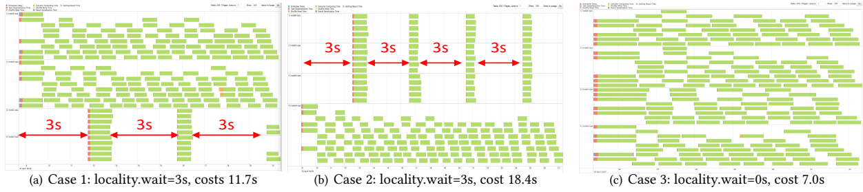
Figure 17: The end-to-end stage latency comparison over different settings for spark.locality.wait.
