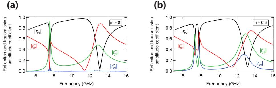
Fig. 3. Calculated spectra of  $|r_{xx}^-|$  (black),  $|t_{xx}^-|$  (red),  $|r_{yx}^-|$  (blue), and  $|t_{yx}^-|$  (green) in a frequency range of 4-16 GHz with (a)  $m = 0$  and (b)  $m = 0.3$ .
