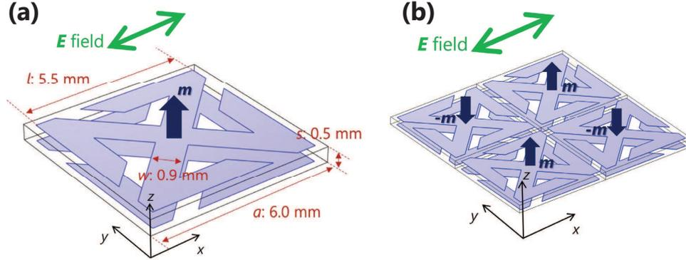
Fig. 2. (a) A unit cell of a calculated MCh metasurface consisting of  $5.5 \text{ mm} \times 5.5 \text{ mm}$  Z-type gammadions on the both sides of a  $0.5 \text{ mm}$ -thick substrate. The substrate is magnetized in the  $+z$  direction. The electric field of the incident microwave is polarized along the  $x$  direction. (b) A unit cell of a calculated composite metasurface including ordinary and contra-position MCh metasurfaces.
