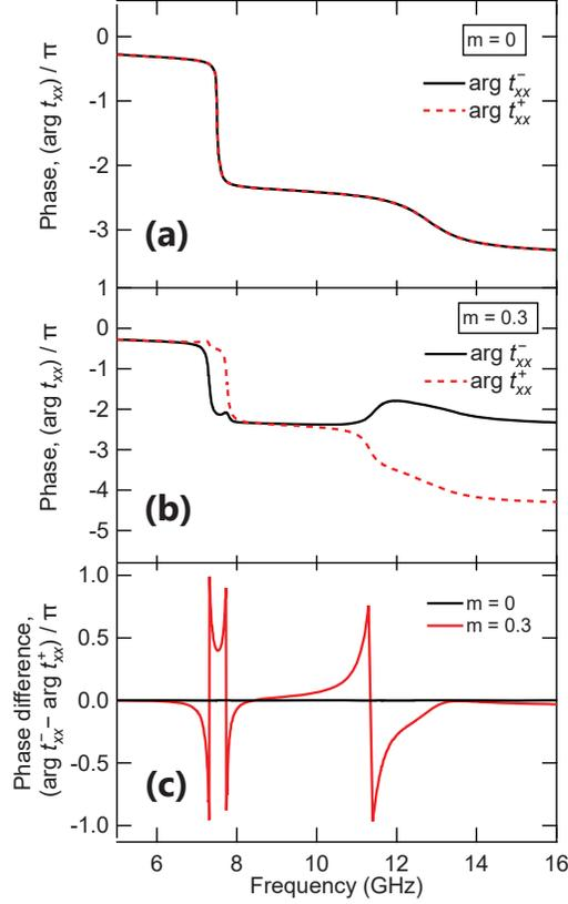
Fig. 4. Calculated spectra of  $(\arg t_{xx}^-)/\pi$  (black solid) and  $(\arg t_{xx}^+)/\pi$  (red dashed) with (a)  $m = 0$  and (b)  $m = 0.3$  in a frequency range of 4-16 GHz. (c)  $(\arg t_{xx}^- - \arg t_{xx}^+)/\pi$  spectra with  $m = 0$  (black) and  $m = 0.3$  (red).
