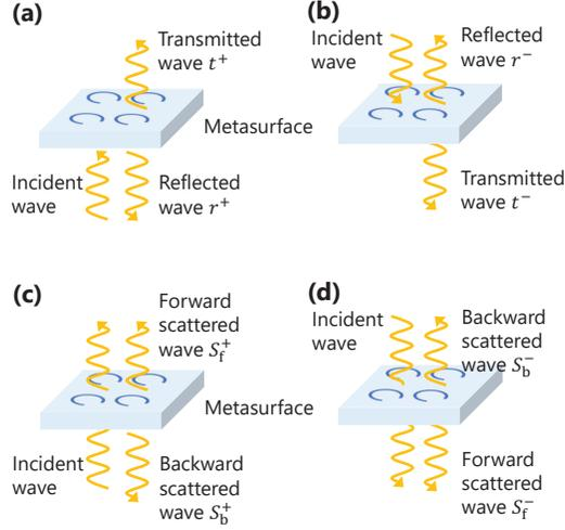
Fig. 1. (a) A transmitted wave  $t^+$  and reflected wave  $r^+$  by the incident wave in the positive direction (+). (b) A transmitted wave  $t^-$  and reflected wave  $r^-$  by the incident wave in the negative direction (-). (c) Redrawn of (a) using the forward scattered wave  $S_f^+$  and the backward scattered wave  $S_b^+$ . (d) Redrawn of (b) using the forward scattered wave  $S_f^-$  and the backward scattered wave  $S_b^-$ .
