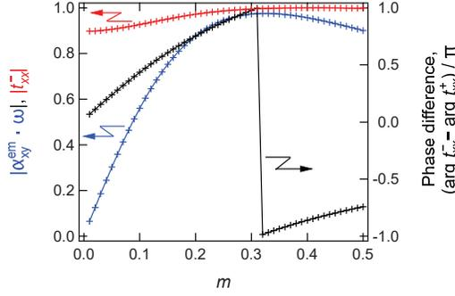
Fig. 9.  $|\alpha_{xy}^{\text{em}}\omega|$  (blue, left axis),  $|t_{xx}^-|$  (red, left axis), and  $(\arg t_{xx}^- - \arg t_{xx}^+)/\pi$  (black, right axis) at 12.0 GHz are plotted as a function of  $m$  from 0 to 0.5.
