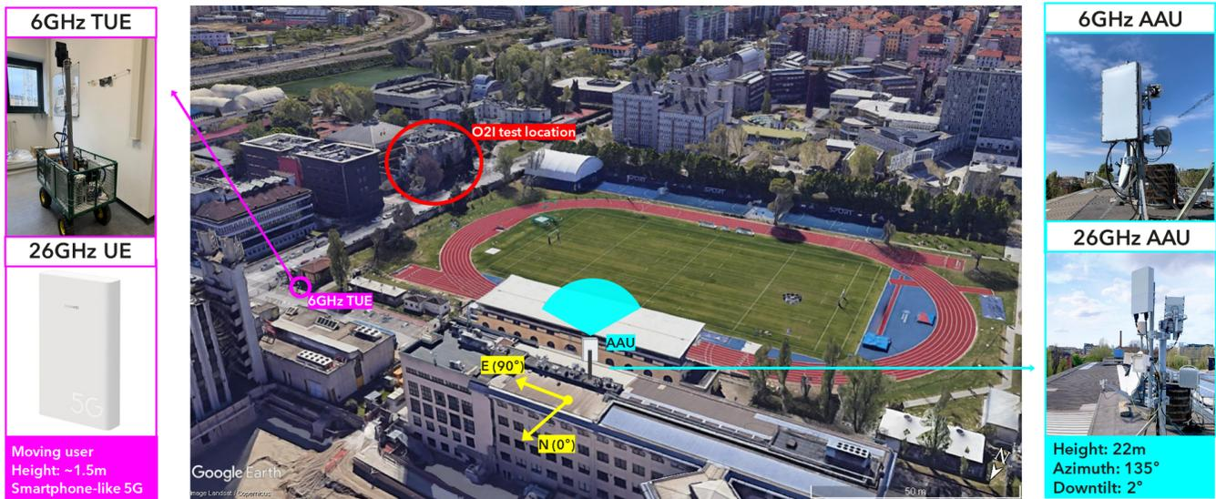
Fig. 1: Aerial view of the test area with equipment details
