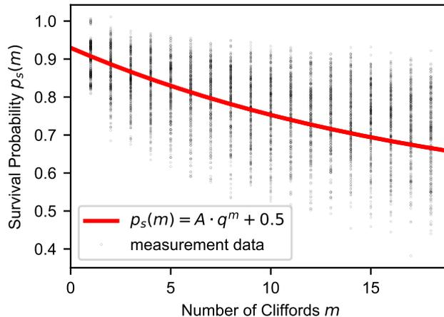
FIG. 3. Randomized benchmarking experiment for an optimized gate-set. The abscissa shows the number of applied Clifford gates  $m$  and the ordinate shows the corresponding survival probability  $p_s(m)$ . The data is fitted using a single exponential decay illustrated by the red line.
