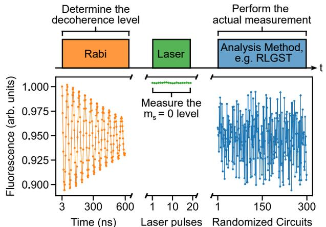
FIG. 6. The measurement sequence for any experiment consists of three parts: a Rabi measurement to determine the decoherence level, a measurement of the  $|0\rangle$  fluorescence level and the actual measurement sequence, e.g. RLGST, which is then converted to expectation values by the previously obtained fluorescence levels.
