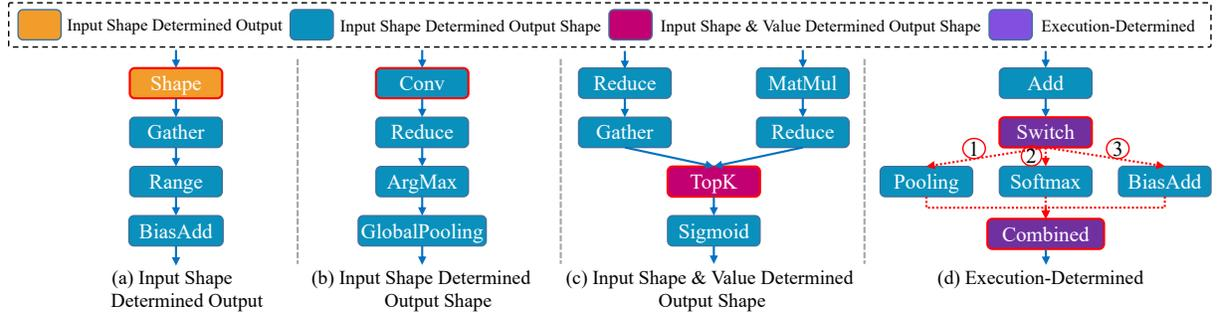
**Figure 1: Different degrees of dynamism.** Each node is a DNN operator. Yellow, blue, red, and purple mean *Input Shape Determined Output*, *Input Shape Determined Output Shape*, *Input Shape & Value Determined Output Shape*, and *Execution Determined Output*, respectively. In (d), Switch’s execution path is decided dynamically during runtime and red dot edges represent both the computation dependency and control flow.
