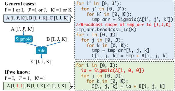
**Figure 4: Operator fusion with dynamic shapes.** The top code snippet shows that fusion is not feasible because of broadcasting [11]. Specifically, *Add* requires  $A$ 's indices  $I'$ ,  $J'$ , and  $K'$  to be either 1 or  $I$ ,  $J$ , and  $K$ , resulting in 8 fusion scenarios. With RDP, such fusion is feasible (shown in the below code snippet). This fusion significantly reduces intermediate result materialization requirements.
