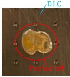
Figure 9: DLC peeling. The orange area in the center has DLC peeling off, exposing the base material polyimide.
