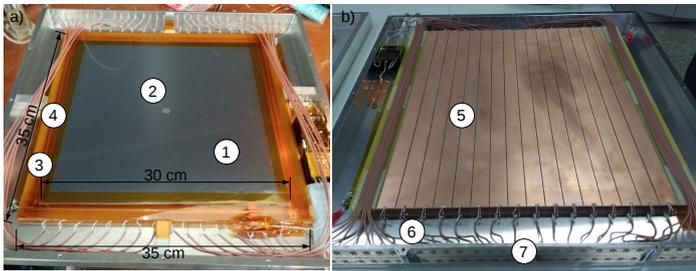
Figure 1: a) sRPC module showing: 1- HV layer, 2- Circular spacer in the center of the active area, 3- Strip spacer all around de the periphery and 4- Mylar™ and Kapton™ layers. b) sRPC plane showing: 5- Readout strip plane, 6- Coaxial cables and 7- MMCX RF feedthrough connectors.
