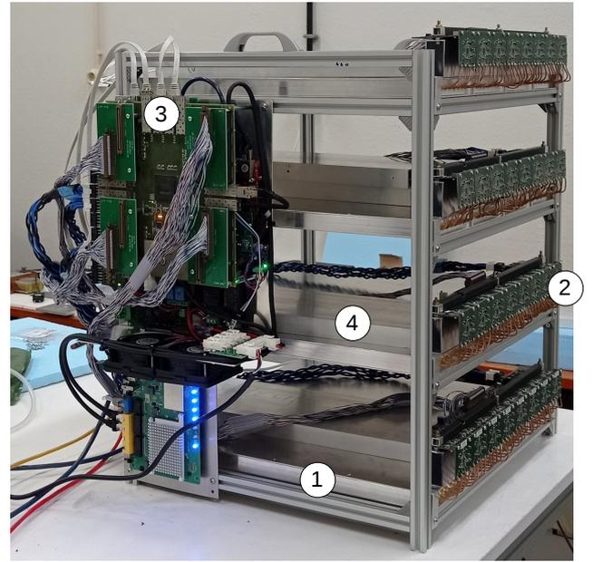
Figure 2: Experimental setup for sRPC characterization consisting of four detection planes equipped with sRPC modules of 300 x 300 mm<sup>2</sup> vertically arranged at a distance of 20 cm. 1- sRPC planes, 2- Fast Front End Electronics board housing 32 channels, 3- DAQ system and 4- HV power supply.
