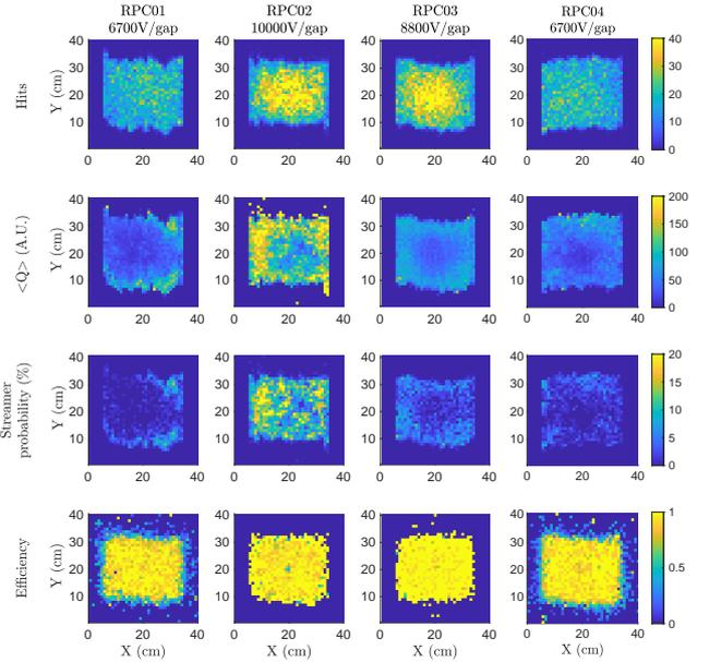
Figure 4: Detected hits, average charge, streamer probability and efficiency for the four planes at a voltages within the HV plateau.
