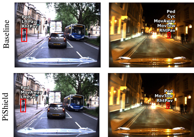
Figure 2: The unconstrained models (top row) violate simple background knowledge rules, predicting (i) that a pedestrian is both on the right and on the left pavement, and (ii) that a person is both a pedestrian and a cyclist, and is moving towards and away from the self-driving vehicle at the same time. On the other hand, the predictions made using PiShield (bottom row) are guaranteed to be compliant with the background knowledge.
