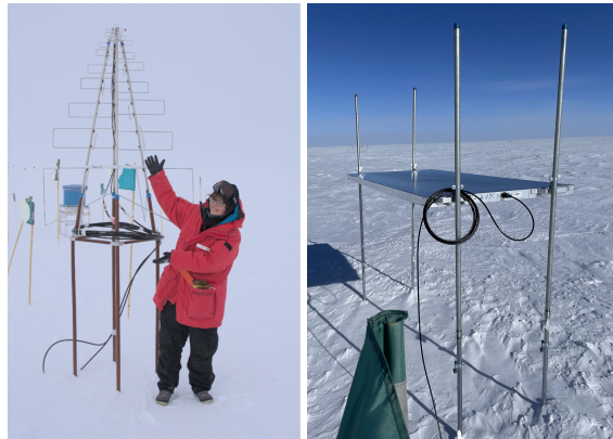
Figure 2: Left: The new deployed antenna with the custom mount; Right: One of the new scintillation detectors.
