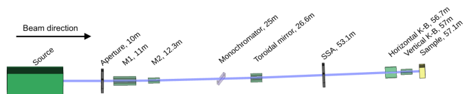
FIG. 4: A schematic of the Tender-Energy X-ray Absorption Spectroscopy (TES, 8-BM) beamline at NSLS-II. This representation shows the many optical components that make up modern beamlines, with each optical component having many degrees of freedom that must be optimized in concert in order to carry out experiments effectively.
