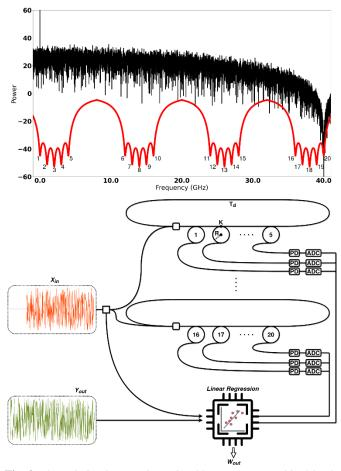
**Fig. 2.** Photonic implementation using 20 MRRs arranged in 4 banks of 5 MRR each that filter the input timeseries. Each MRR is centered on a specific part of the input spectrum (inset – black), denoted by the corresponding number on the combined transfert function of the MMRs (inset – red).
