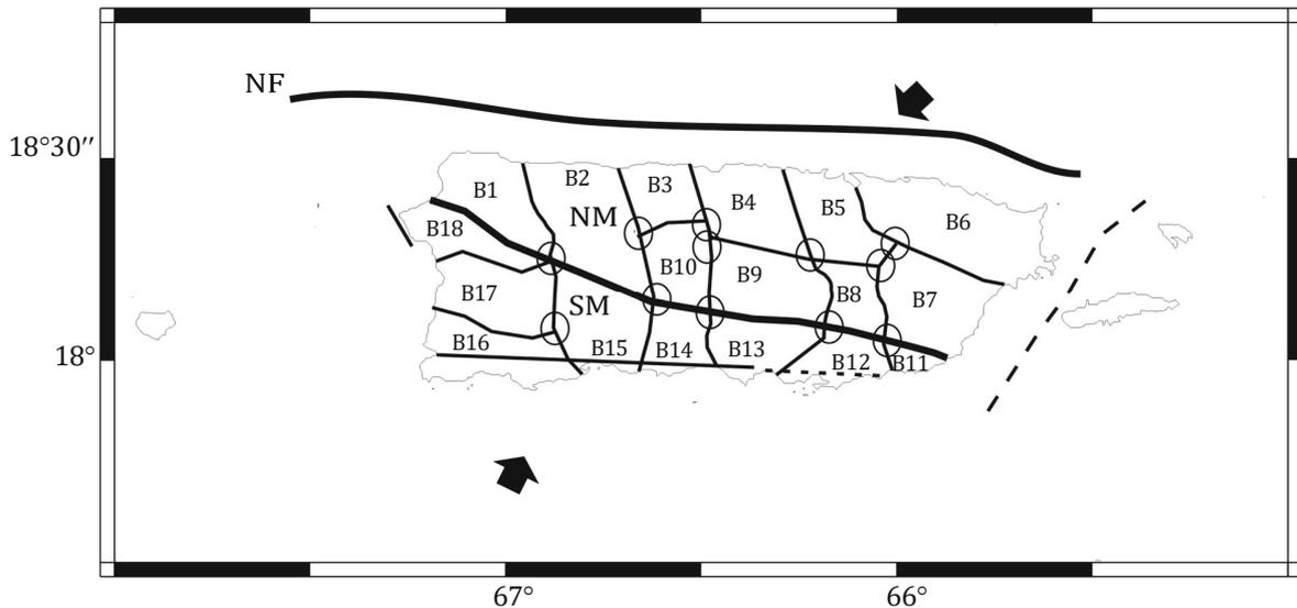
**Fig. 7.** Morphotectonic map of Puerto Rico. Black arrow is the main direction of movement; black circle, knot; black lines, alignments of faults: NF—Northern; curve black arrow, direction of block movement; mesoblocks: NM—Northern, SM—Southern.
