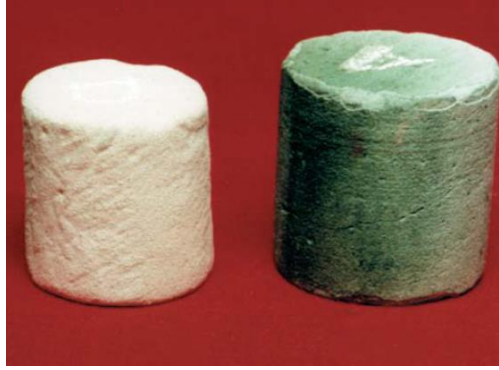
Figure 2. A visual comparison of ThermaLock cement (right) and Portland cement (left) under CO 2 exposure.
