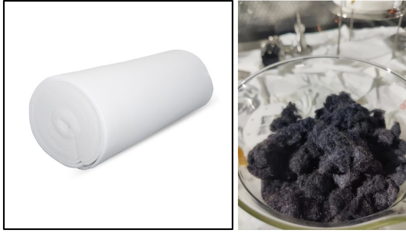
Figure 1: Pictures of polyurethane fiber (left) and Mn-fiber (Right).
