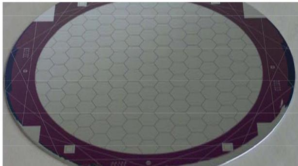
Figure 5-2: The Nab experiment silicon detector (back side).
