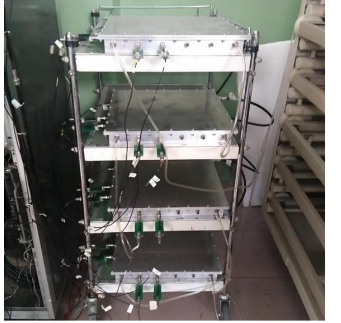
FIG. 12. Prototype of muon imaging system based on delay line readout and glass RPC developed by Peking University.
