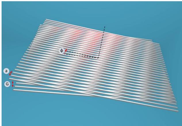
**Figure 1:** Schematic representation of the twist-controlled double-layer wire metasurface (DLWM) structure.
