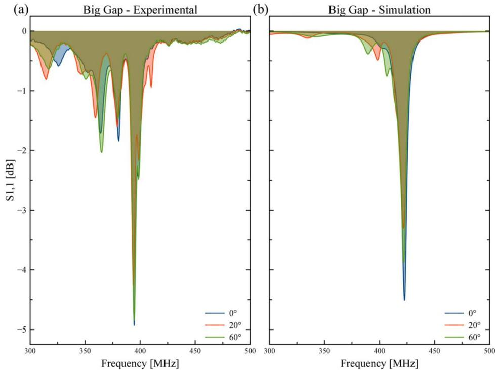
**Figure 4:** Reflection coefficient ( $S_{11}$ ) analysis for the DLWM structure with a big gap. (a) Experimental measurements showing the original resonance frequency's minor change upon relative rotations for a big gap ( $G = \sim 30\text{ mm}$ ). (b) Simulated results for a big gap ( $G = 10\text{ mm}$ ) confirming the experimental findings.
