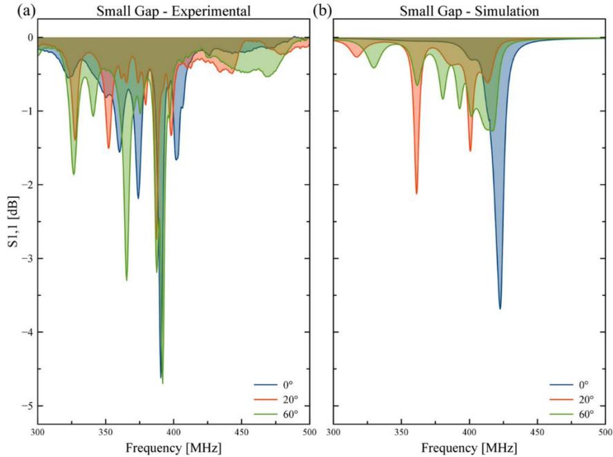
**Figure 3:** Experimental and simulated reflection coefficient ( $S_{11}$ ) analysis of the DLWM structure. (a) Measured  $S_{11}$  values for a small gap ( $G = 5\text{mm}$ ) at 0°, 20°, and 60° rotations, illustrating the main resonance frequency around 390 MHz and its subsequent splitting and shift towards lower frequencies with rotation. (b) Full-wave simulation results for a small gap ( $G = 2\text{mm}$ ) at the same rotational condition.
