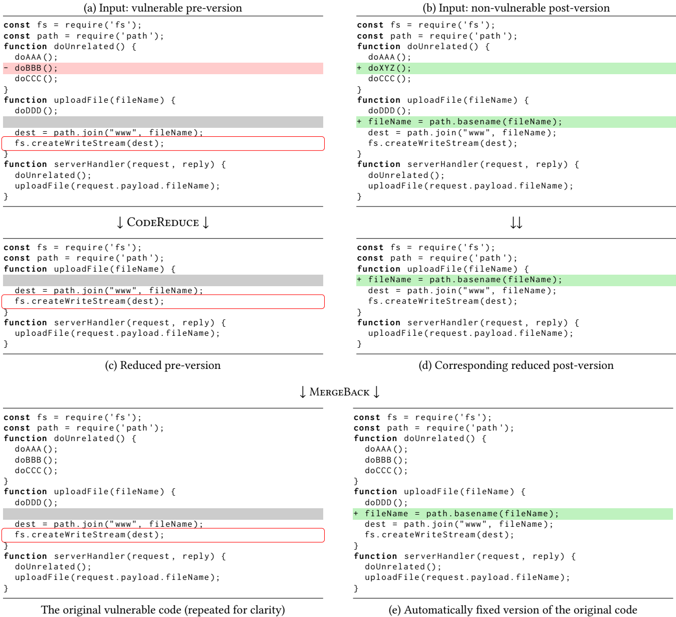
Figure 2. An example run of our data creation pipeline on a diff containing a path traversal vulnerability [37] fix (a)→(b). Colors: red -/green +/gray represent standard diff notation, and framed line marks the location of the vulnerability. CODEREDUCE is applied on (a), and a similar transformation is then applied on (b) to get (d), whereas MERGEBACK is applied to obtain (e) from (a) and the diff of (c)→(d). Other real-world fix examples generated fixes by DEEPCODE AI FIX can be found in Appendix C.
