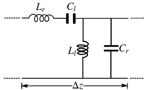
FIG. 1. Schematic diagram of equivalent unit-cell circuit of the quantized CRLH-TL.
