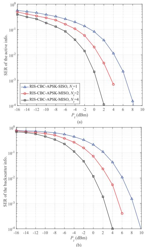
Fig. 9. Performance of passive RIS-CBC-APSK in SISO and MISO scenarios, where  $A = P = 4$  and  $N_t = 1, 2, 4$ .
