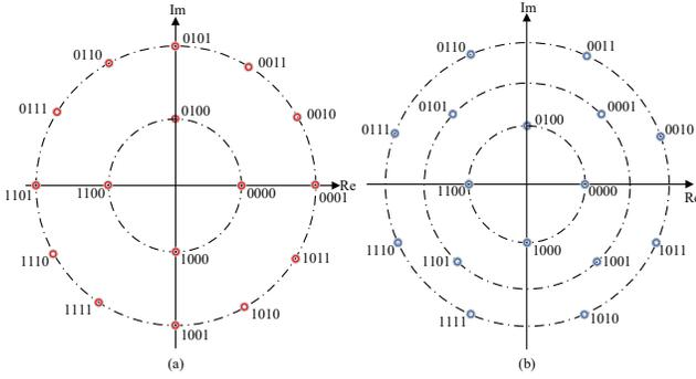
Fig. 1. Examples of 16-APSK constellations: (a) 4 + 12-APSK and (b) 4 + 4 + 8-APSK.
