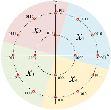
Fig. 4. The partition for 4 + 12-APSK with  $A = P = 4$ .
