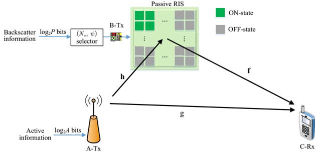
Fig. 2. Block diagram of passive RIS-CBC-APSK in a SISO setting.
