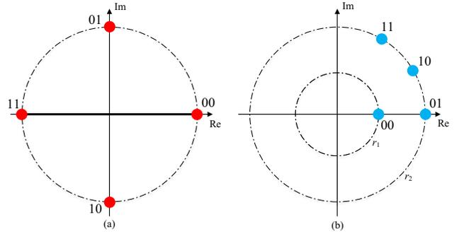
Fig. 3. Constellations of (a)  $x$  and (b)  $\mathcal{H}_{N_a} e^{j\psi}$ , for  $A = P = 4$ .
