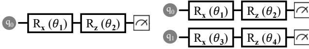
Figure 2: Overview of quantum classifier circuits: The left figure shows a one-qubit classifier circuit for a two-dimensional dataset (Fig. 1 left), while the right figure depicts a two-qubit classifier circuit for a four-dimensional dataset (Fig. 1 right).
