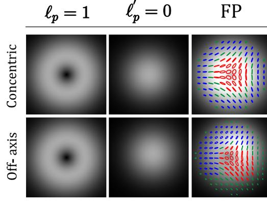
**Figure 4.** This figure illustrates the effect of imperfect overlap between the two constituent LP modes of an FP mode. In the upper row we show the ideal case involving two concentric modes giving rise to an ideal FP beam (third column). The bottom row shows the effect of a slight non-concentricity between the two constituent LP modes, leading to a noticeable polarization distribution deformation. The colormap is as the shown in Figures 2 and 3
