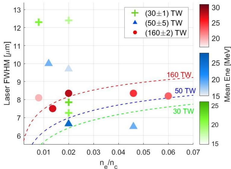
**Figure 3.** The scattered markers show the experimental data in the [ laser FWHM – plasma density ] domain. Green plus markers are obtained using laser power of  $(30 \pm 1)$  TW, blue triangles are obtained using laser power of  $(50 \pm 5)$  TW and red dots are obtained using laser power of  $(160 \pm 2)$  TW. The color darkness indicates the electron mean energy, with darker color representing higher energy.
