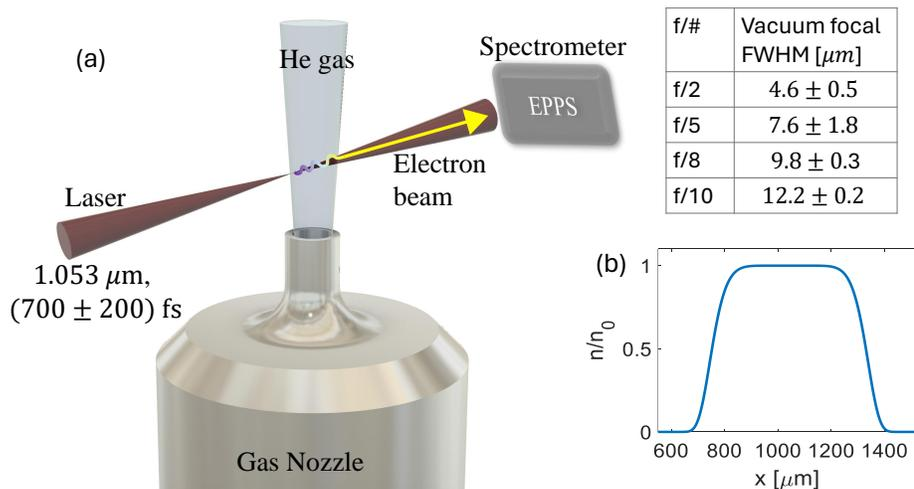
**Figure 1.** (a) Experimental setup. The table on the right shows  $f$ -number for four different apodizers and the corresponding in-vacuum laser FWHM. (b) The longitudinal density profile in simulations.  $n_0$  is the peak plasma density, which is  $0.02 n_c$ .
