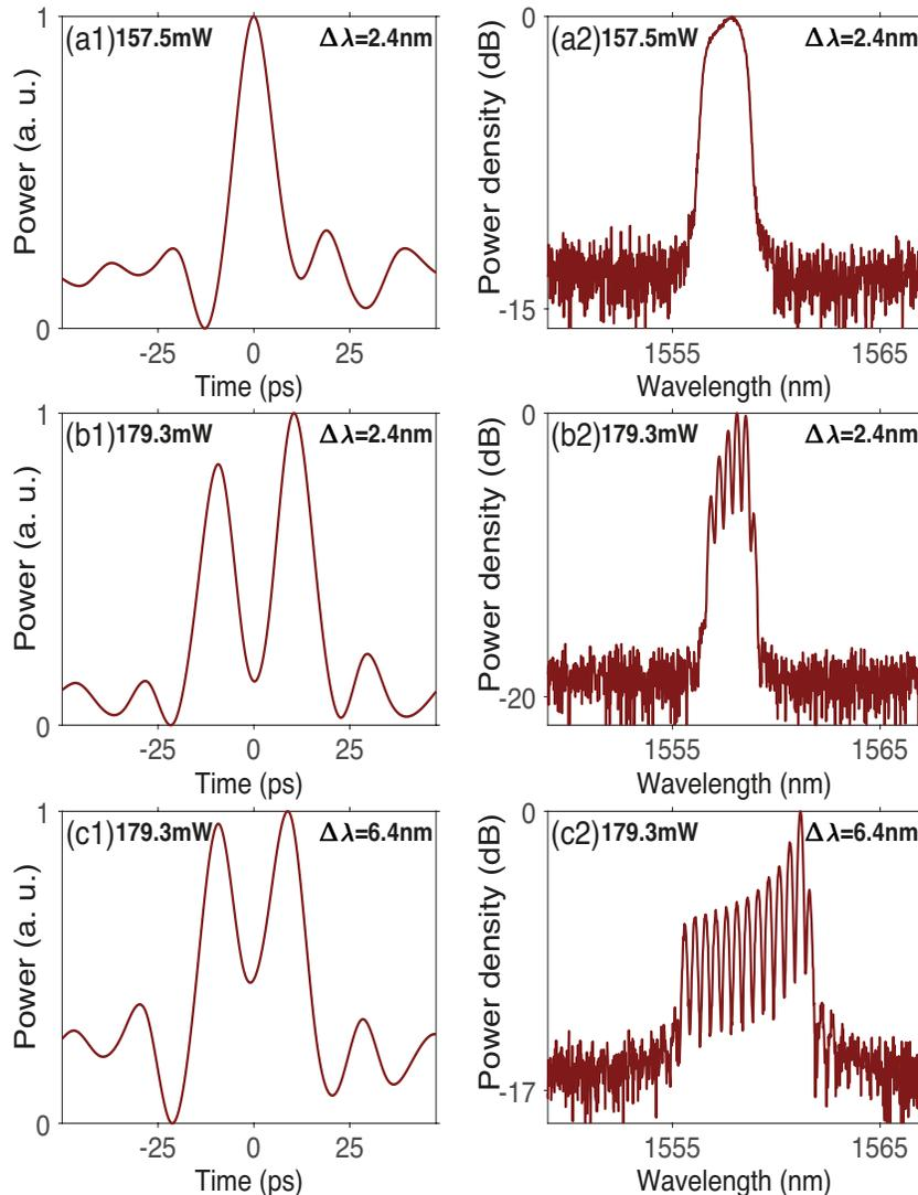
Figure 8: Temporal and spectral profiles of the structures generated at the three main steps of the 2D procedure illustrated in Fig. 7. (a1)-(a2): structure obtained just above the mode-locking threshold. (b1)-(b2): structure obtained at the intermediate point (II). (c1)-(c2): structure obtained at the end point (F).
