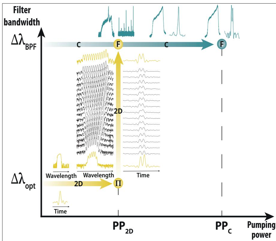
Figure 7: Experimental results showing access to multi-pulse regime by the conventional procedure (path labeled "C") and the 2D-OT (path labeled "2D").  $\Delta\lambda_{opt}=2.4\text{nm}$ .  $\Delta\lambda_{BPF}=6.4\text{nm}$ .  $PP_{2D}=179.3\text{mW}$ .  $PP_C=338\text{mW}$ .
