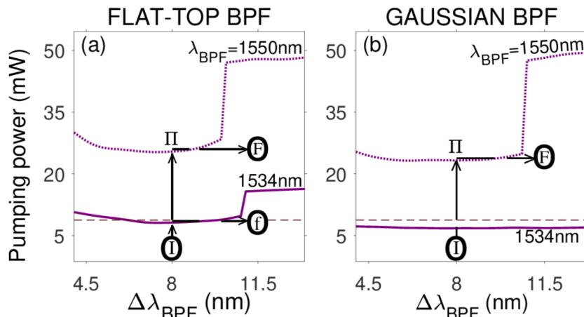
Figure 2: Fragmentation pumping power vs filter bandwidth, for a cavity with 1.55 $\mu\text{m}$ -centered BPF (dotted curves) and 1.534 $\mu\text{m}$ -centered BPF (solid-line curves). The dashed horizontal line corresponds to the FPP for the BPF-free cavity.
