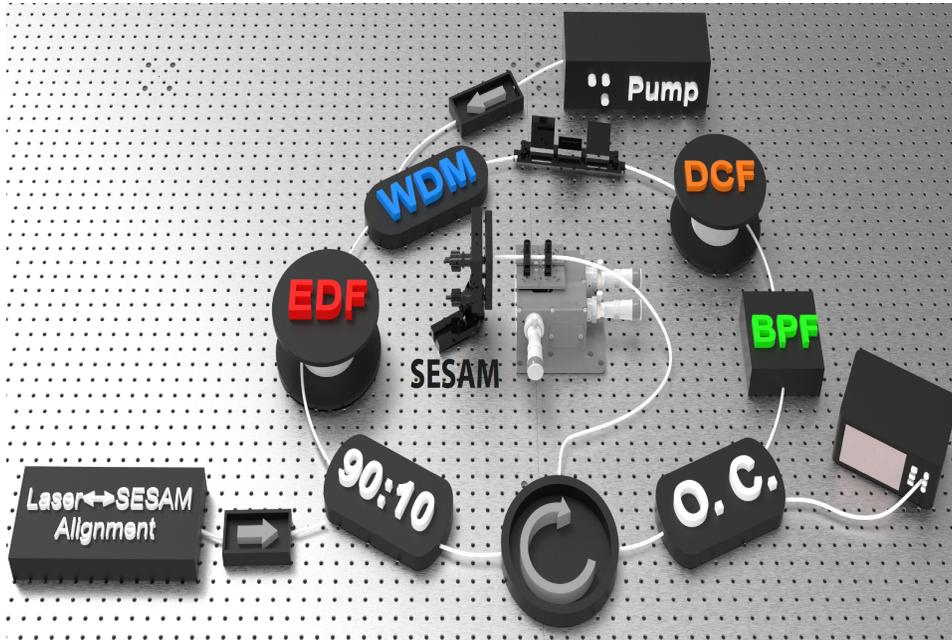
Figure 6: Experimental setup of the laser cavity. Intensity profile and spectra are respectively measured with an optical spectrum analyser and a 63 GHz oscilloscope.
