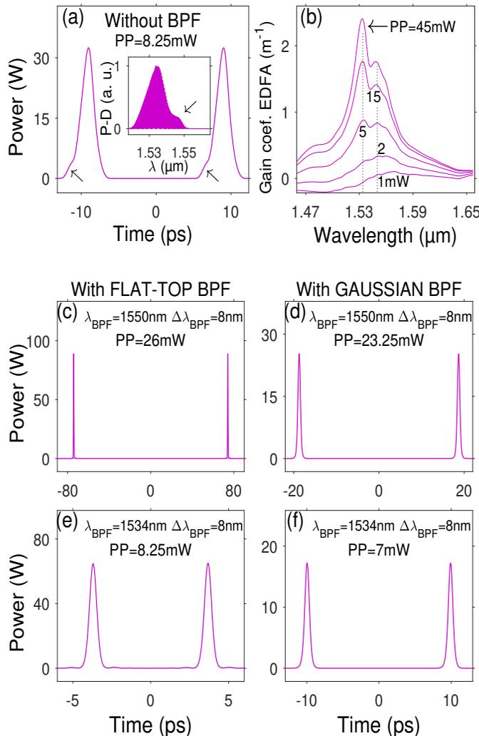
Figure 3: Intensity profiles just after pulse fragmentation, recorded at the output of the OC2, in the region where  $\Delta\lambda_{BPF} < \Delta\lambda_c$ . (a): Pulse temporal profile for the BPF-free cavity. The inset shows the spectral power density (P-D). (b) : Gain coefficient of the EDFA. (c), (d), (e), and (f) : Temporal profiles in presence of BPF with  $\Delta\lambda_{BPF}=8\text{nm}$ .
