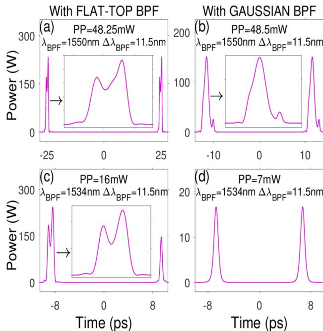
Figure 4: Intensity profiles just after pulse fragmentation, for  $\Delta\lambda_{BPF} = 11.5nm$ .
