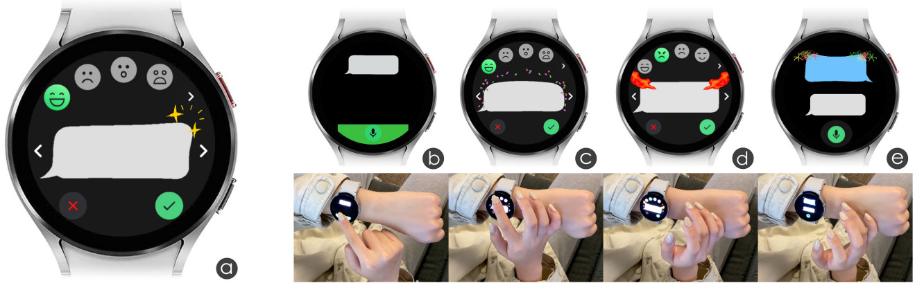
Figure 1: (a) EmoWear is a smartwatch voice messaging system enabling users to apply 30 animated emotional teasers: pre-retrieval cues offering a glimpse into an awaiting message’s emotional tone before diving into the audio content; EmoWear interaction flow typically includes: (b) recording the message, (c,d) browsing and selecting emotional teasers, (e) receiving the message.
