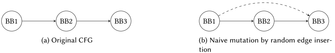
Fig. 2. An example showing that naive mutation of CFG may break domination relations. Figure 2a shows the original CFG. If we randomly insert an edge shown in Figure 2b, BB2 won't dominate BB3 after mutation, and any value in BB3 referencing BB2 becomes invalid.
