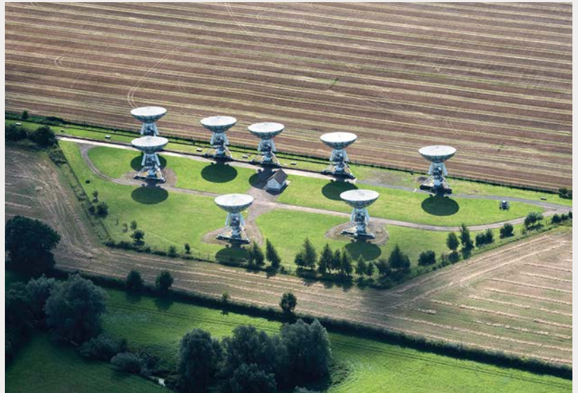
A1 Aerial view of the AMI-LA array in Cambridge, UK. The longest baseline is 110m. This telescope has for many years performed high-cadence follow-up of a wide range of astrophysical transients and variables. AMI-LA is operated by the University of Cambridge. (John Fielding Aerial Images)
