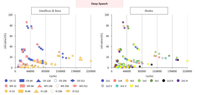
Fig. 14. The number of cycles and utilization values for all systolic array configurations under the DeepSpeech workload.
