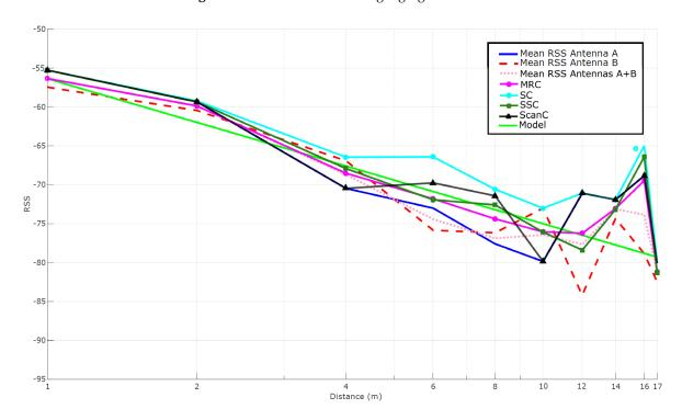
Figure 18. RSS means and multi-antenna techniques when using high-gain antennas.
