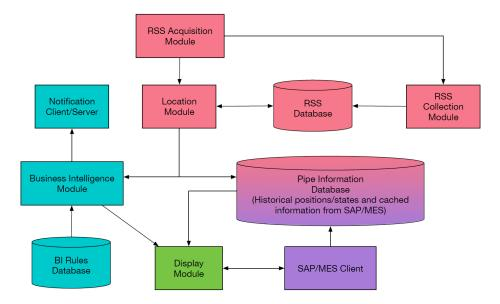
**Figure 6.** Modules of the smart pipe system proposed.
