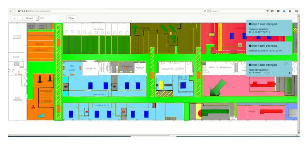
Figure 23. Notifications shown on the right upper part when a pipe crosses from one area to another.
