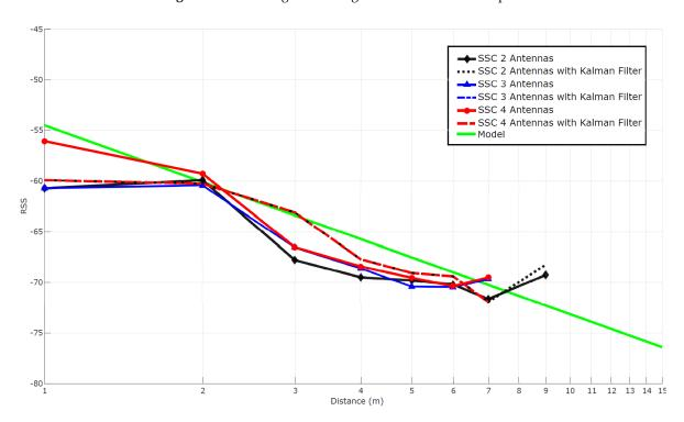
Figure 13. Stabilizing Exo 800 tag RSS with the SSC technique.
