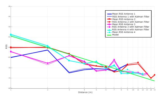
Figure 10. Exo 800: Comparison of the RSS curves with and without Kalman filtering.
