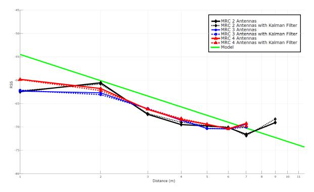
Figure 11. Stabilizing Exo 800 RSS with the MRC technique.
