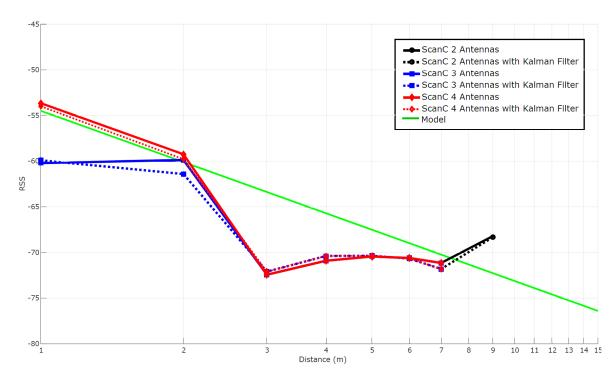
Figure 14. Stabilizing Exo 800 tag RSS with the ScanC technique.
