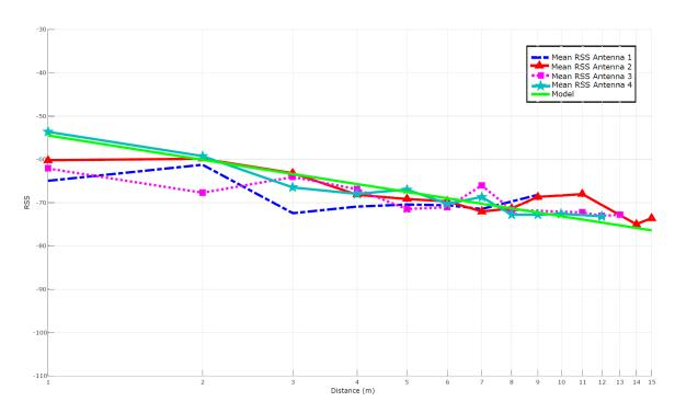
**Figure 9.** Exo 800: mean curves for each antenna and model obtained with the mean of the four antennas.
