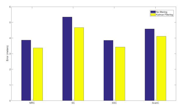
Figure 20. Multi-antenna technique stability with and without Kalman filtering.
