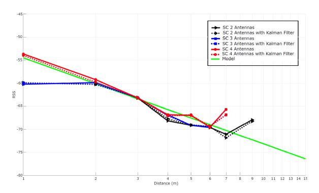
Figure 12. Stabilizing Exo 800 tag RSS with the SC technique.
