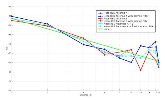
Figure 19. Comparison of the RSS curves when using Kalman filtering in the active system.
