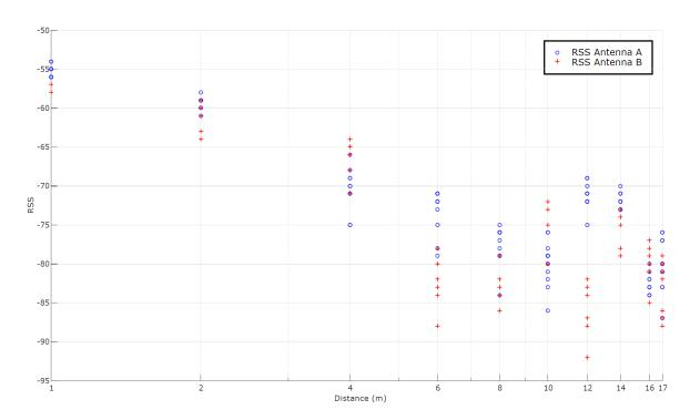
Figure 17. RSS values when using high-gain antennas.
