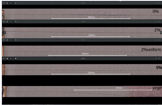
Fig. 9 Optical microscopy snapshots for anode wires irradiated with 5, 2, 0% \text{CF}_4 gas mixtures compared to a virgin sample.
