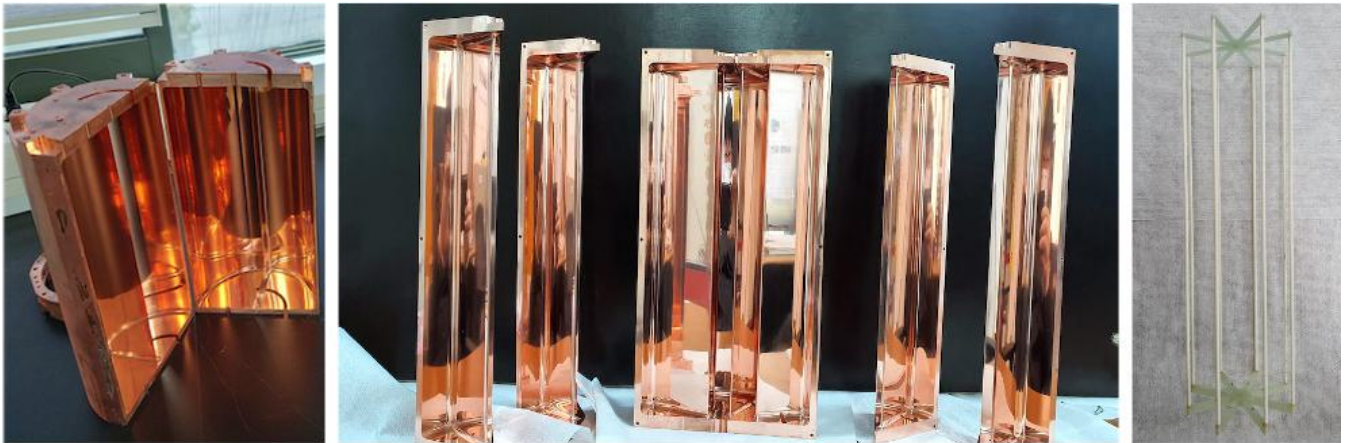
Figure 2. Photographs of individual pieces of the 2-cell and 8-cell cavities used for the experiments described in the text. The tuning structure for the 8-cell cavity is also shown.
