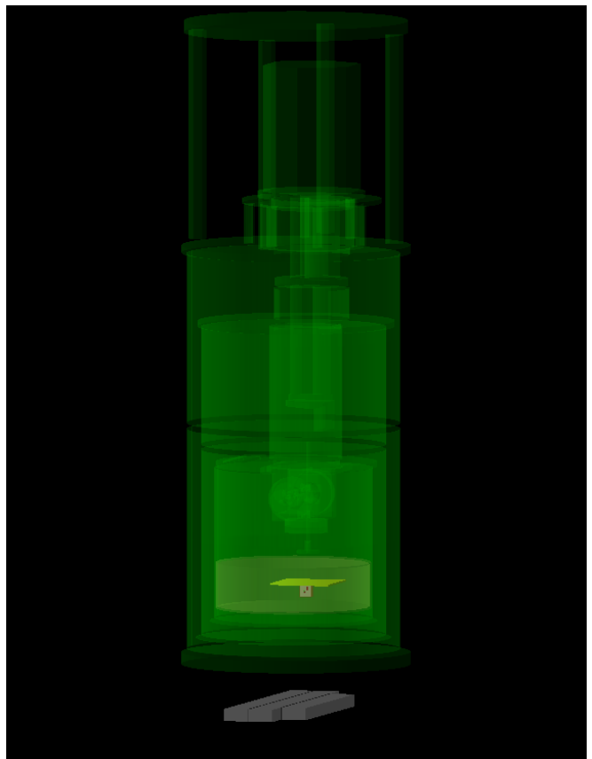
FIG. 10. GEANT4 graphic user interface output of Sim 4. It includes the ADR, the 30 mK-plate, the magnetic shield, the copper box housing the TES substrates, and, in gray, the three sabers below the refrigerator.
