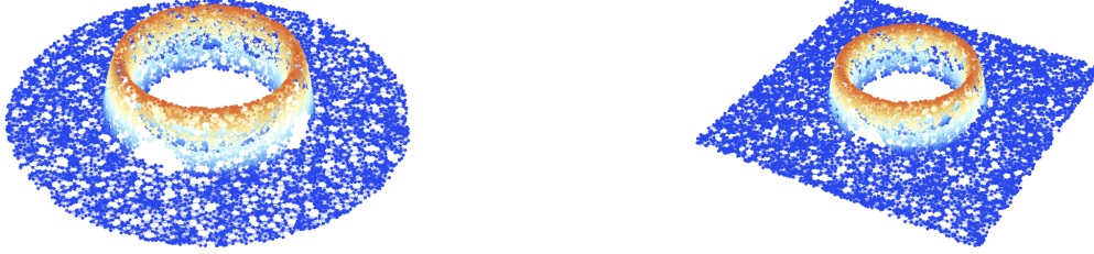
Figure 11: On the left, the final ( t = 100M ) hypersurface configuration for the radial accretion of an initially spherically-symmetric fluid distribution onto an uncharged, non-rotating black hole in Schwarzschild/spherical polar coordinates (t, r, \theta, \phi) , with a resolution of 10,000 hypergraph vertices (colored based on fluid density), and with both spatial coordinate and fluid density coordinate information assigned to the vertices. On the right, the final ( t = 100M ) hypersurface configuration for the radial accretion of an initially spherically-symmetric fluid distribution onto an uncharged, non-rotating black hole in Kerr-Schild/Cartesian coordinates (t, x, y, z) , with a resolution of 10,000 hypergraph vertices (colored based on fluid density), and with both spatial coordinate and fluid density coordinate information assigned to the vertices.
