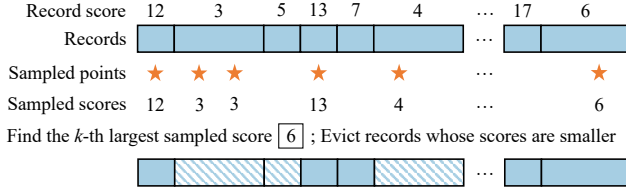
Figure 4: Eviction in RALT. Each record has a score shown above it, and the length represents its size (HotRAP size or physical size). The sampled points are shown as stars in this virtual size space.
