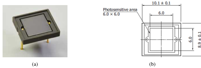
Figure 1: (a) Image of the S13370–6075CN SiPM model tested in this work. (b) Dimensional outline [mm]
