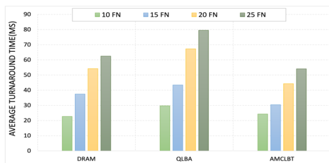
Figure 11. Comparison of average turnaround time for DRAM, QLBA, and AMCLBT using different number of fog nodes 10, 15, 20, and 25 executing homogeneous tasks
